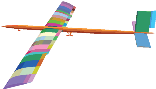
Fig. 14 Aircraft flutter mode at trimmed level flight.
